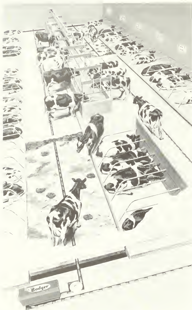
Figure 3.5.14 Reversing alley scraper (courtesy Badger Northland Inc.)
